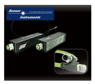
Sensors from Sensor Instruments, which have an RS232 interface, can be connected via converters to the appropriate programmable logic controllers (PLCs).
